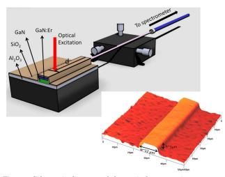
Fig. 3. Schematic diagram of the optical attenuation measurement setup and an AFM image of the GaN:Er waveguide fabricated based on sample A4 (GaN:Er/GaN/Al<sub>2</sub>O<sub>3</sub>) with waveguide width  $w \sim 12 \ \mu m$  and height  $h \sim 1 \ \mu m$ .
