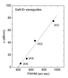
Fig. 5. Optical attenuation coefficient of GaN:Er waveguides as a function of the GaN (002) XRD rocking curve linewidth measured from four different structures: A1 (GaN:Er/GaN/AlN/Al\_2O\_3), A2 (GaN:Er/GaN/Al\_{0.75}Ga\_{0.25}N/AlN/Al\_2O\_3), A3 (GaN/GaN:Er/GaN/Al\_2O\_3), and A4 (GaN:Er/GaN/Al\_2O\_3).
