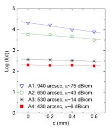
Fig. 4. Optical attenuation measurement results obtained from GaN:Er waveguides fabricated based on four different structures: A1 (GaN:Er/GaN/All\_O\_3), A2 (GaN:Er/GaN/Al\_{0.75}Ga\_{0.25}N/AlN/Al\_2O\_3), A3 (GaN/GaN:Er/GaN/Al\_2O\_3), and A4 (GaN:Er/GaN/Al\_2O\_3). The solid lines are the least-squares fit of data using Eq. (2).
