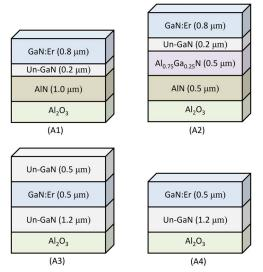
Fig. 1. Schematic structure diagrams of four different GaN:Er samples: A1 (GaN:Er/GaN/AlN/Al<sub>2</sub>O<sub>3</sub>), A2 (GaN:Er/GaN/Al<sub>0.75</sub>Ga<sub>0.25</sub>N/AlN/Al<sub>2</sub>O<sub>3</sub>), A3 (GaN/GaN:Er/GaN/Al<sub>2</sub>O<sub>3</sub>), and A4 (GaN:Er/GaN/Al<sub>2</sub>O<sub>3</sub>).
