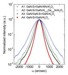
Fig. 2. GaN (002) XRD rocking curves measured from four different GaN:Er samples: A1 (GaN:Er/GaN/Aln/Al<sub>2</sub>O<sub>3</sub>), A2 (GaN:Er/GaN/Al<sub>0.75</sub>Ga<sub>0.25</sub>N/Aln/Al<sub>2</sub>O<sub>3</sub>), A3 (GaN/GaN:Er/GaN/Al<sub>2</sub>O<sub>3</sub>), and A4 (GaN:Er/GaN/Al<sub>2</sub>O<sub>3</sub>).
